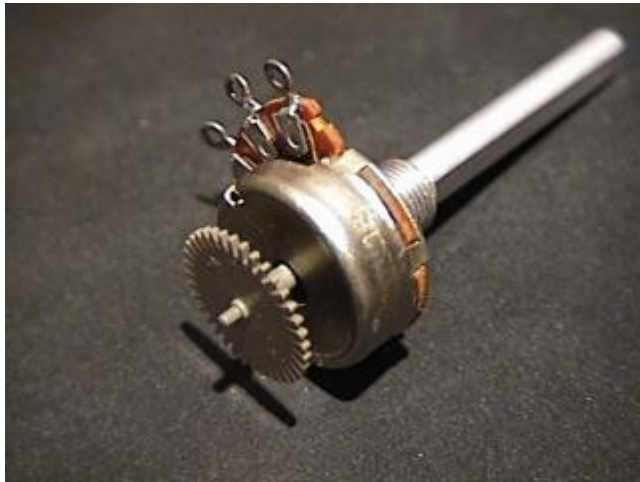
Figure 6 - Encoder fitted to potentiometer
