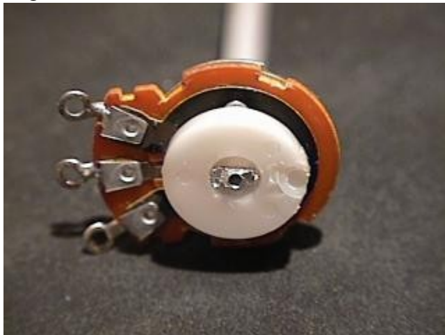
Figure 4 - Shaft center hole and stopper removed.
